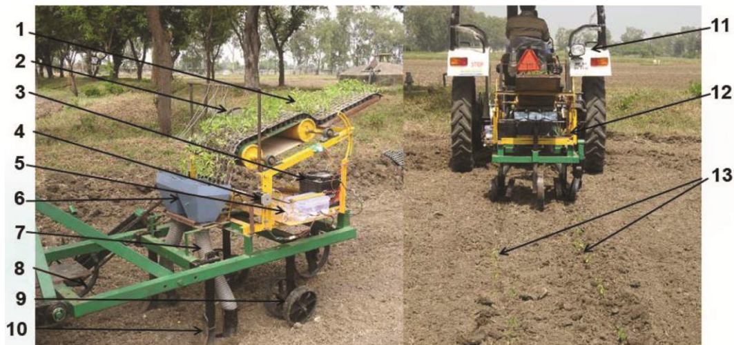
Fig. 4 — Developed automatic vegetable transplanter with its components (1-Seedling pro-tray; 2-DC motor; 3-Battery 12V; 4-Stepper motor; 5-Microcontroller based system; 6-Delivery box; 7-Delivery pipe; 8-Ground wheel; 9-Press wheel; 10- Furrow opener; 11-Tractor; 12-Developed transplanter; 13-Transplanted seedlings)
