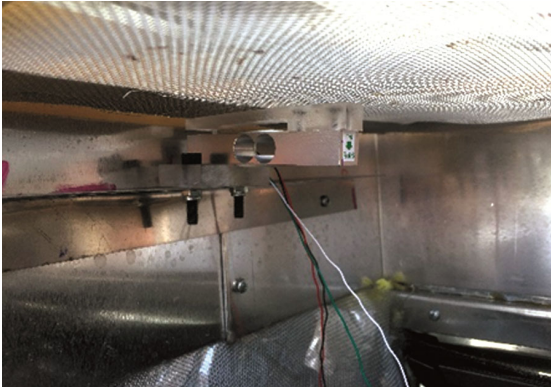
Fig. 6 — The view of a load cell mounted on a rack
