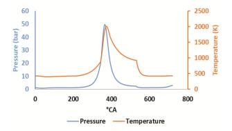
Fig. 4 — Pressure and Temperature vs CA
