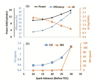
Fig. 10 — Influence of spark advance on (a) Efficiency, Power and SFC; (b) NO and CO  $\,$
