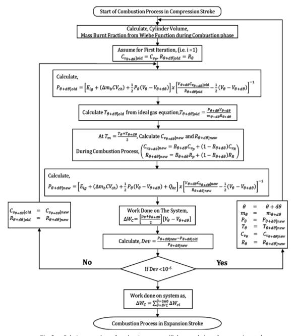
Fig. 2 — Solution procedure of combustion process till the completion of compression stroke
