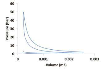
Fig. 5 — P-V diagram for producer gas engine
