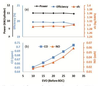
Fig. 13 — Influence of exhaust valve opening (EVO) on (a) Efficiency, Power and SFC;(b) NO and CO Fig. 11(b)
