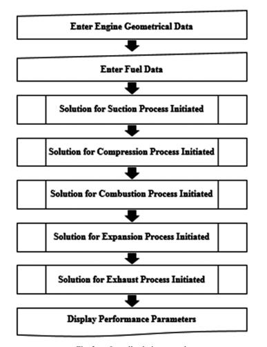
Fig. 3 — Overall solution procedure
