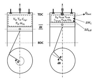
Fig. 1 — Control volume of combustion process during compression stroke before and after 'd $\theta$ ' interval of crank angle
