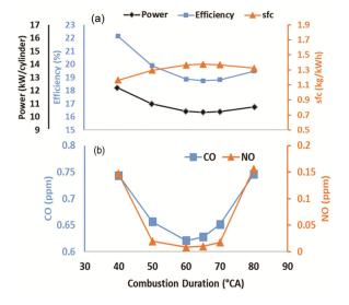
Fig. 11 — Influence of combustion duration on (a) Efficiency, Power and SFC (b) NO and CO
