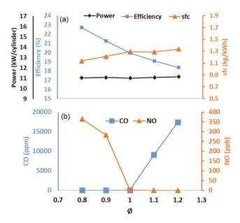
Fig. 7 — Influence of fuel-air ratio ( $\emptyset$ ) on (a) Efficiency, Power and SFC; (b) NO and CO emission
