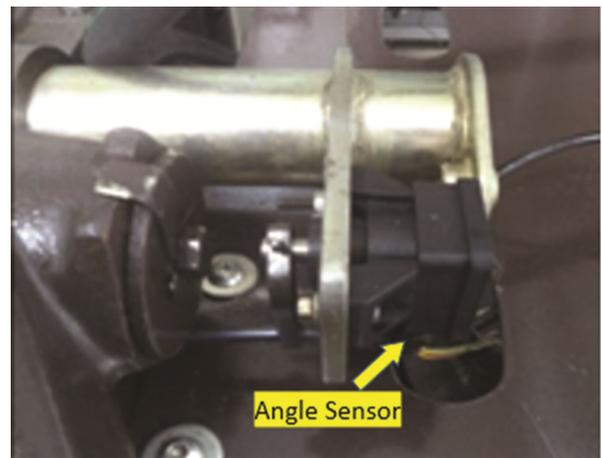
Fig. 5 — Placement of angle sensor
