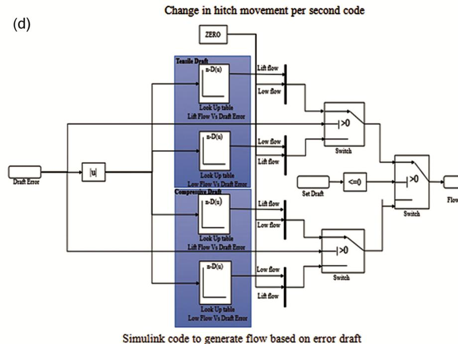
Fig. 7 — MATLAB simulink code: (a) Overall draft control code, (b) Change in sensed force per second code, (C) Change in hitch movement per second code, (d) Simulink code to generate flow based on error draft
