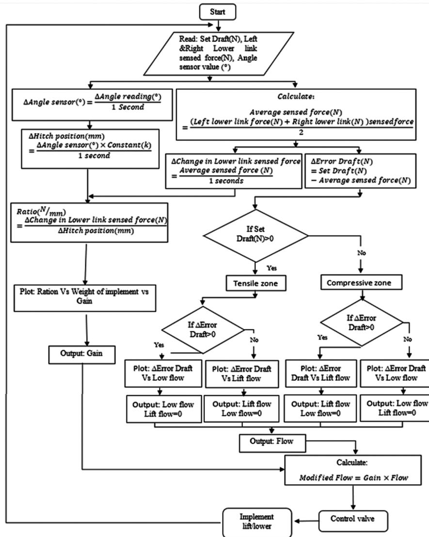
Fig. 6 — Control algorithm of EHH system through lower link draft sensing
