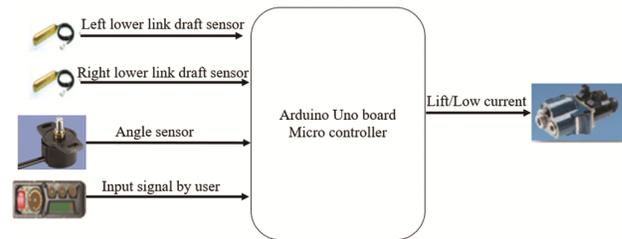
Fig. 1 — EHH systems through lower links draft sensing architecture
