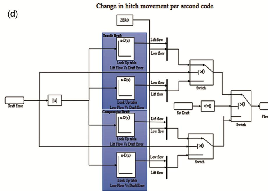
Simulink code to generate flow based on error draft
