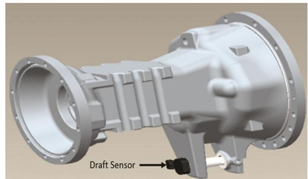
Fig. 4 — Isometric view for position of the draft sensor
