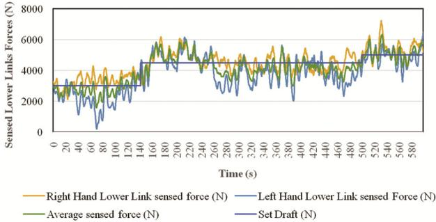
Fig. 9 — Variation of sensed lower link force with time
