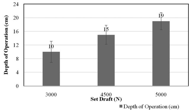
Fig. 12 — Depth of operation with set draft variation
