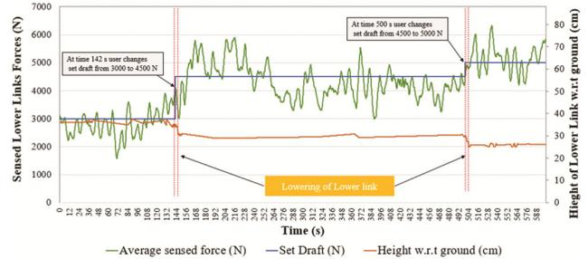
Fig. 11 — Performance and response time of the developed system
