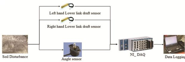
Fig. 8 — Instrumentation set up
