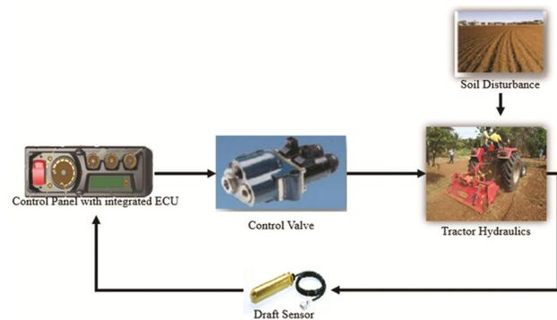
Fig. 2 — EHH system using lower links draft sensing as a closed loop system
