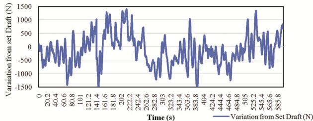
Fig. 10 — Variation of sensed force from set draft with time
