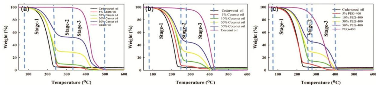
Fig. 4 — Comparison of TGA patterns of cedarwood oil: pure, and adulterated using 5%, 10%, 30% and 50% of (A) Castor Oil, (B) Coconut Oil, and (C) PEG-400
