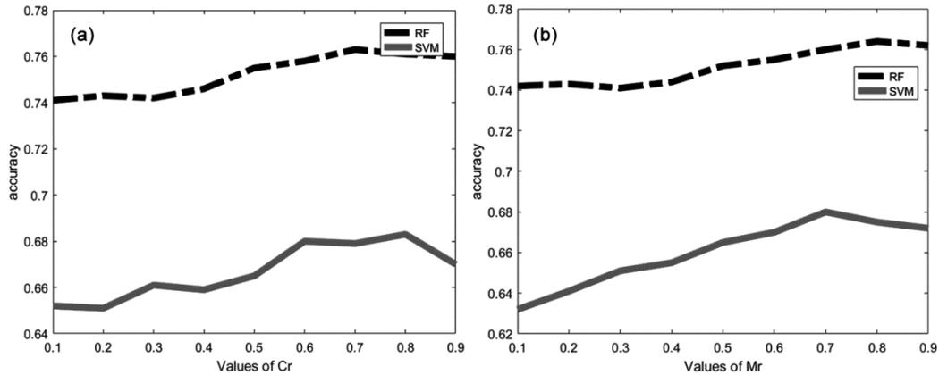
Fig. 2 — (a) Accuracy of RF and SVM plotted against different values of ‘ $C_r$ ’ for dataset-1; (b) Accuracy of RF and SVM plotted against different values of ‘ $M_r$ ’ for dataset-1
