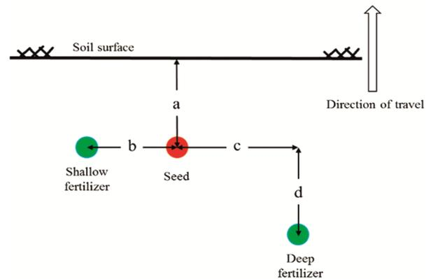
Fig. 1 — Position of seed and fertilizer in dual banding system (a) seed placement depth, (b) lateral placement of shallow fertilizer from seed, (c) lateral placement of deep fertilizer from seed, (d) deep fertilizer placement depth from seed
