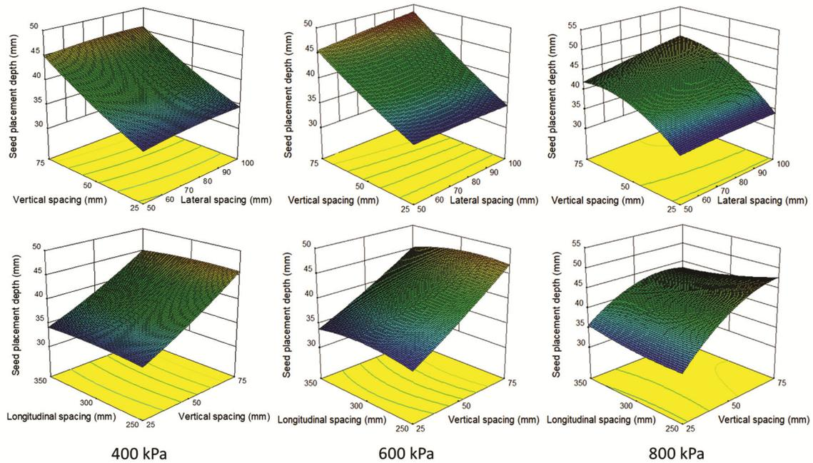
Fig. 10 — Effect of tines spacing on seed placement depth at different soil compactions levels
