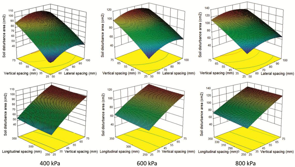
Fig. 7 — Effect of tines spacing on soil disturbance area at different soil compactions levels
