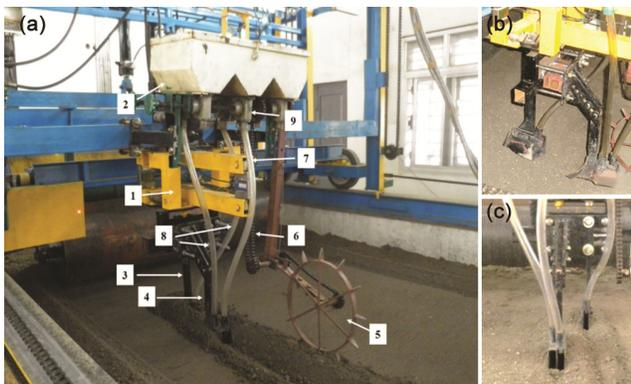
Fig. 3 — (a) Laboratory experimental setup for dual banding fertilizer application, (b) side view of dual tine, (c) back view of dual tine. (1) Force measuring unit, (2) Seed and fertilizer box, (3) fertilizer tine, (4) Shallow tine, (5) Ground wheel, (6) Chain drive, (7) Seed tube, (8) Fertilizer tubes, (9) Metering unit
