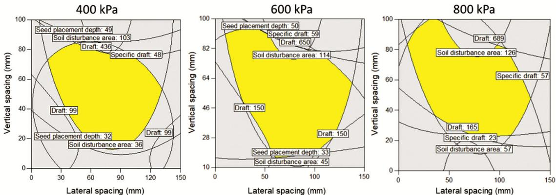
Fig. 11 — Overlay plot of lateral and vertical spacings at optimized longitudinal spacing for different soil compaction levels
