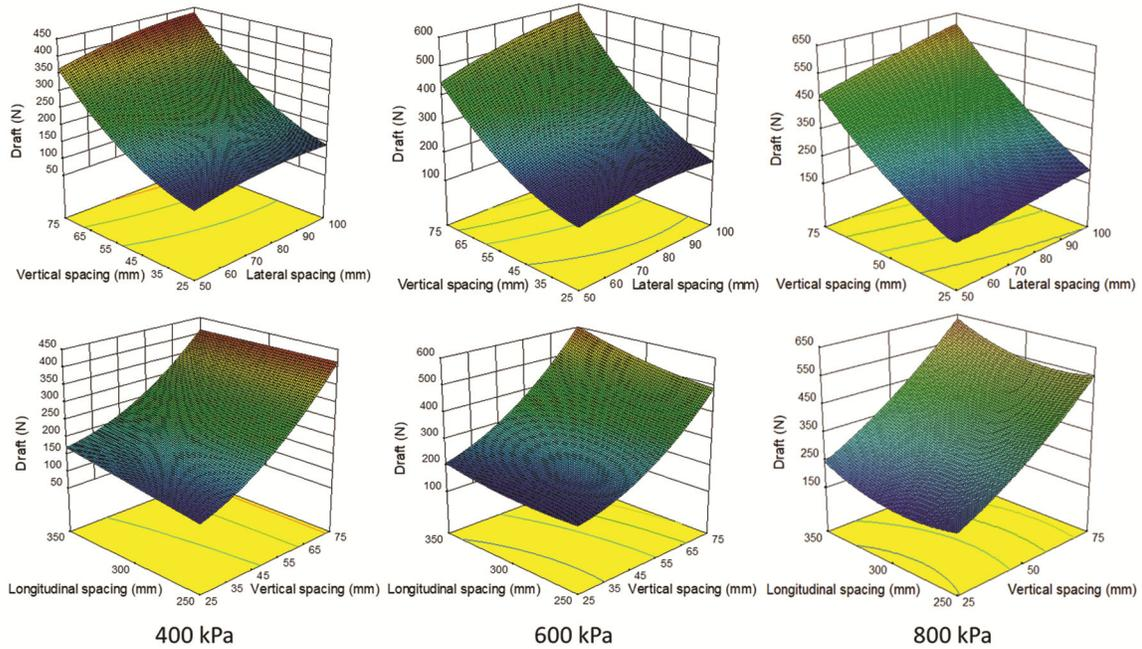
Fig. 5 — Effect of tines spacing on draft at different soil compactions levels
