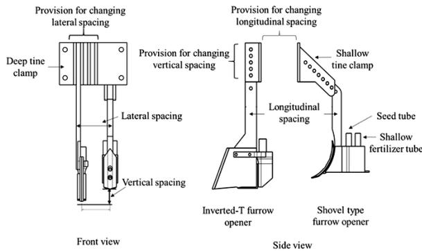
Fig. 2 — Arrangement of dual tines used for band placement of fertilizer
