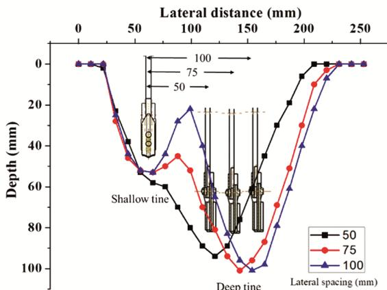
Fig. 8 — Soil disturbance caused by dual tine at different lateral spacing, 50 mm vertical spacing and 300 mm longitudinal
