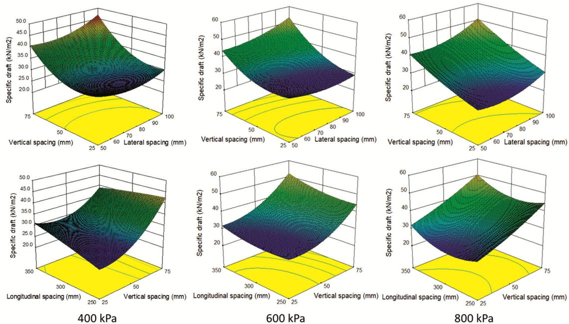
Fig. 9 — Effect of tines spacing on specific draft at different soil compactions levels
