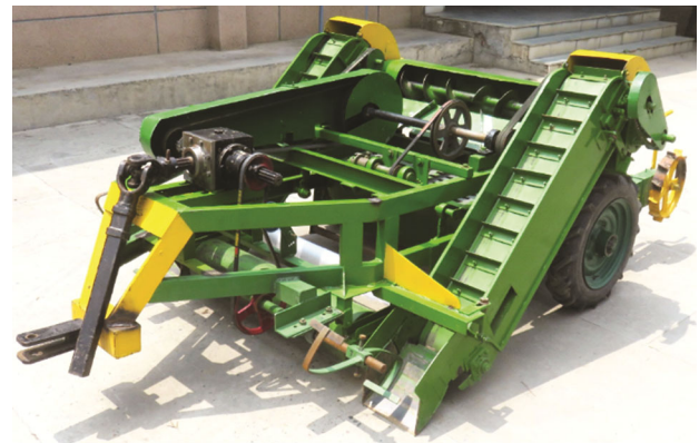
Fig. 5 — A stationary view of developed/assembled tractor-operated seeder for mat type nursery
