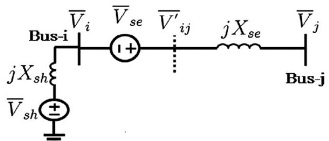
Fig. 1 — UPFC representation using voltage sources.
