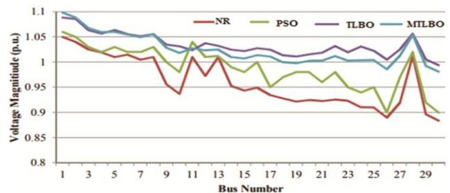
Fig. 3 — Voltage profile improvement with FACTS devices
