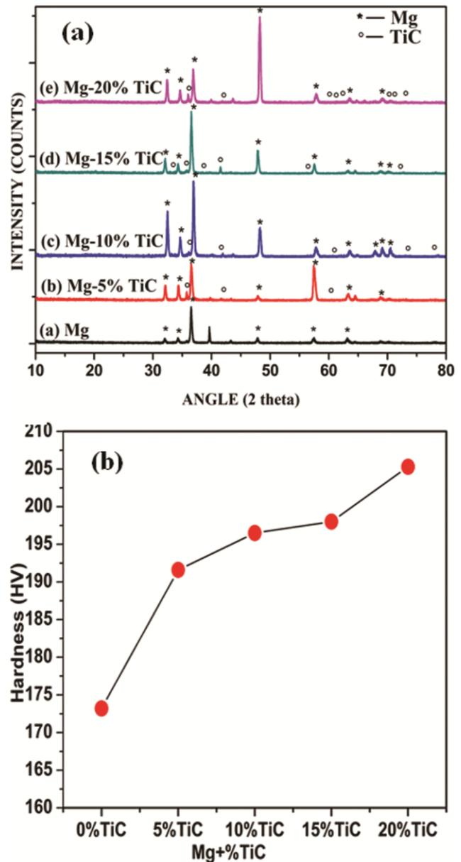
Fig. 2 — XRD of Mg /TiC and influence of TiC on hardness of Mg alloy (a) XRD of various composite from 0-20 wt% TiC (b) and influence of TiC on hardness
