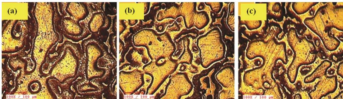
Fig. 1 — Optical Micrograph of 100X magnification of (a) Mg alloy (b) Mg-15% TiC(c) Mg-20% TiC composites
