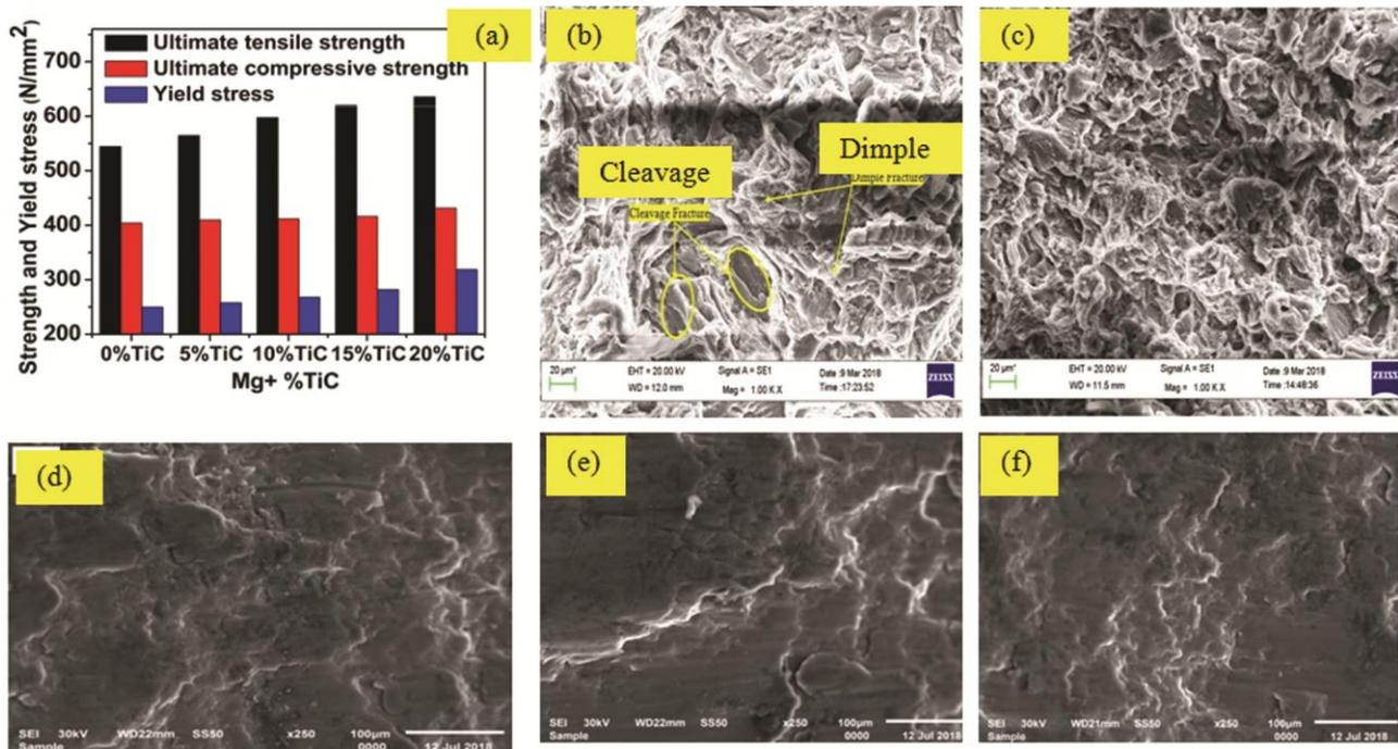
Fig. 3 — Influence of %TiC on strength and SEM images of tensile and compressive fracture surface (a) Influence of %TiC on strength (b)&(c) Tensile of 0%TiC, 20%TiC respectively (d),(e)&(f) compressive of 0%TiC, 15%TiC,20%TiC respectively
