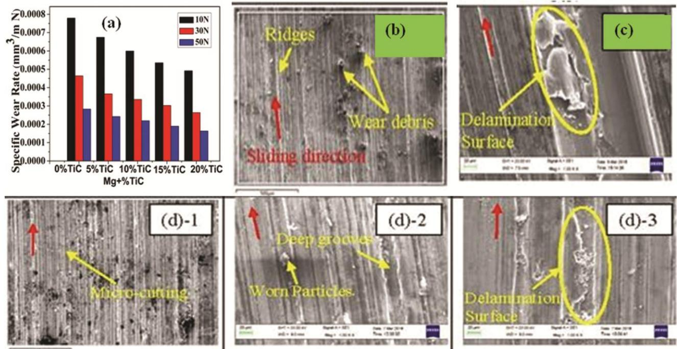
Fig. 4 — Influence of %TiC on wear and SEM images of worn surfaces during various load (a) Influence of %TiC on wear (b)&(c) worn surface 0%TiC at 10 & 50N respectively (d-1), (d-2)&(d-3) worn surface 20%TiC at 10, 30, 50N respectively
